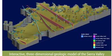
Interactive, three-dimensional geologic model of the Sierra Valley groundwater basin used to define the boundaries and parameterization for the integrated hydrologic model.
