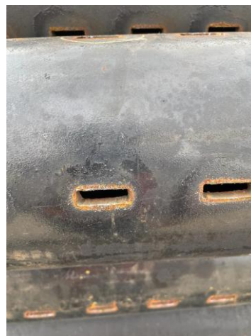
Figure 5. Example of laser cut pre-perforated casing
