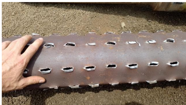
Figure 4. Example of perforated casing section with in-situ perforator
